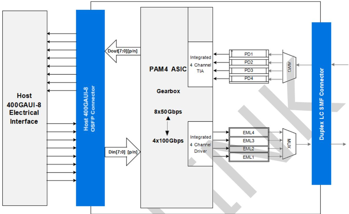
Figure 1: Transceiver Block Diagram
